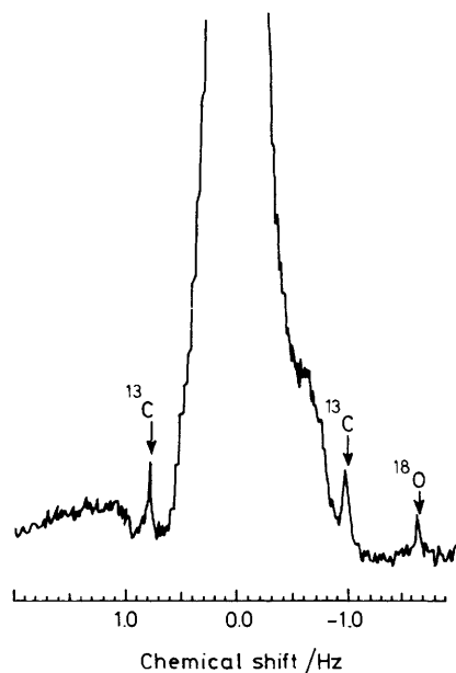
Figure 1. A region of \pm 2 Hz relative to the major resonance in the ultrahigh resolution ^{29}\text{Si} n.m.r. spectrum of \text{Me}_3\text{SiOMe} (with 20% v/v, \text{C}_6\text{D}_6 in a 10 mm sample tube) acquired with the INEPT sequence and noise modulated broad-band proton decoupling on Bruker WM-360 spectrometer at 71.55 MHz and 303 K. ^{13}\text{C} and ^{18}\text{O} Satellites of the OMe group are visible. Number of scans 80, spectral width 300 Hz, acquisition time 27.3 s, 16 K data points acquired. The data were processed with 30 mHz Lorentzian narrowing plus \text{GB} = 0.4 and zero-filling into 128 K data points, which yielded a digital resolution of 4.5 mHz.
